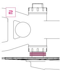
It is important that you use the supplied spacers to preload the bearings correctly. A different number of spacers is provided depending on the width.
