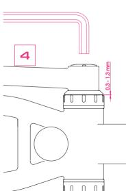
Finally, the left crank including the screw is fitted onto the spindle. The crank bolt must be tightened with an 8mm allen key and 25 Nm.
