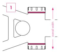
First, install the bottom bracket according to the manufacturer's instructions. Then measure the width of the installed bottom bracket. The width must be between 92.5-95.5mm.
