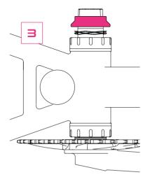
The wave spring and the compression ring must now be pushed onto the spindle. Check clearance between chainring and chainstays.
