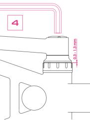
Finally, the left crank including the screw is fitted onto the spindle. The crank bolt must be tightened with an 8mm allen key and 25 Nm.
