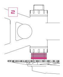
It is important that you use the supplied spacers to preload the bearings correctly. A different number of spacers is provided depending on the width
