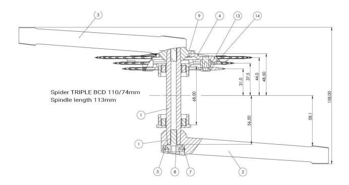
The square of the inner bearing should be clean and free of grease. To fit the cranks, use an 8 mm Allen key and tighten the screw to max. 25 Nm. A higher tightening torque can damage the integrated puller. The square of the inner bearing should be clean and free of grease. After approx. 50 km of riding, please check the fit of the crank bolt and retighten if necessary.
